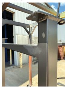
is coming out blotchy around some of the welded ioint areas after curing, but also shows up in some of the straight areas of the tubing. We did prime these parts with a gel cure and neither the substrate nor
