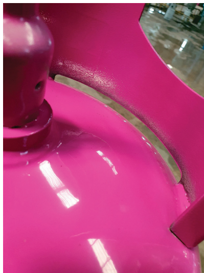
Poor powder coverage in handle area of gas cylinder.
