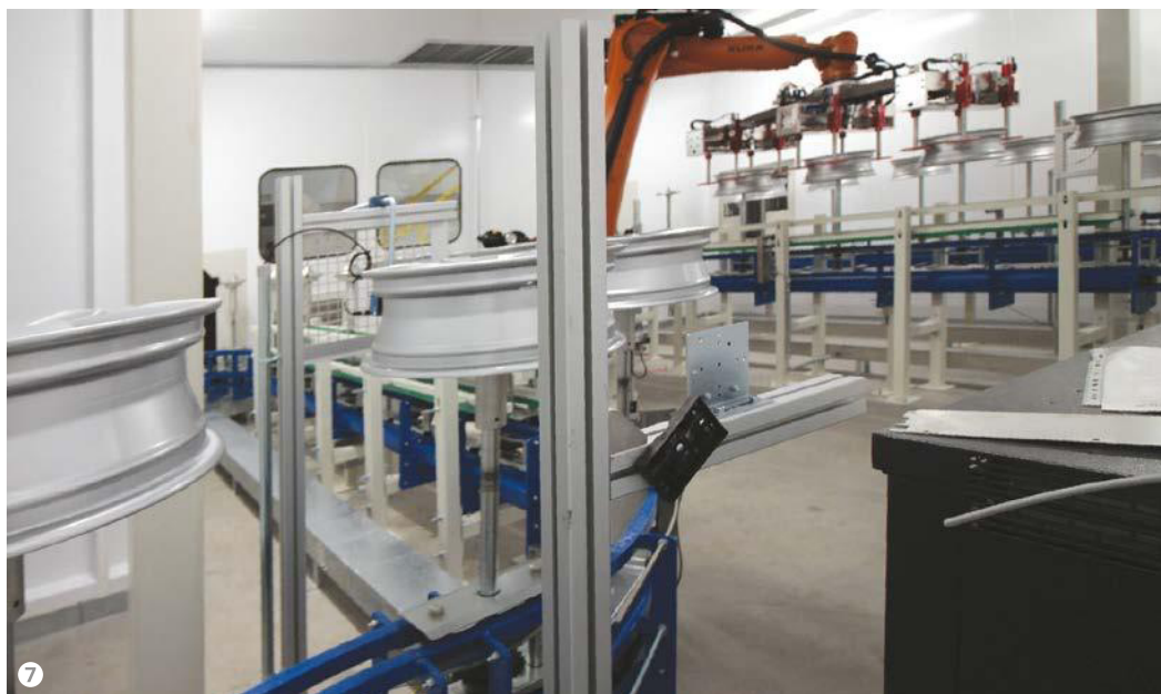
Figure 7: The robotic transfer from the powder application circuit to the liquid application one.
