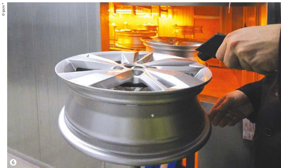
Figure 6: A sample check of the wheel temperature after passing into the IR pre-heating chamber.
