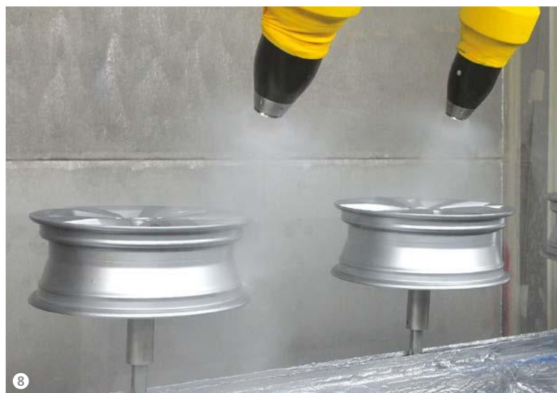
Figure 8: The base coat and clear coat are applied with EcoBell2 Dürr electrostatic technology.
