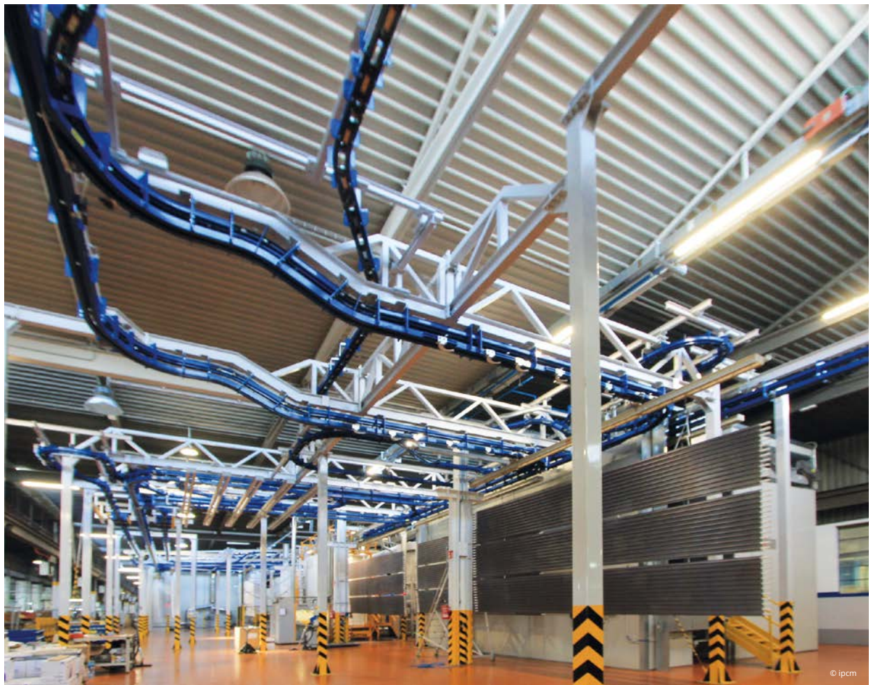
After passing through the drying oven and the cooling area, the parts move on to the powder application booth.
