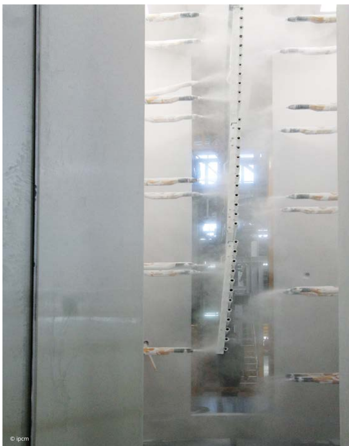
Powder coating application with dense phase technology.
