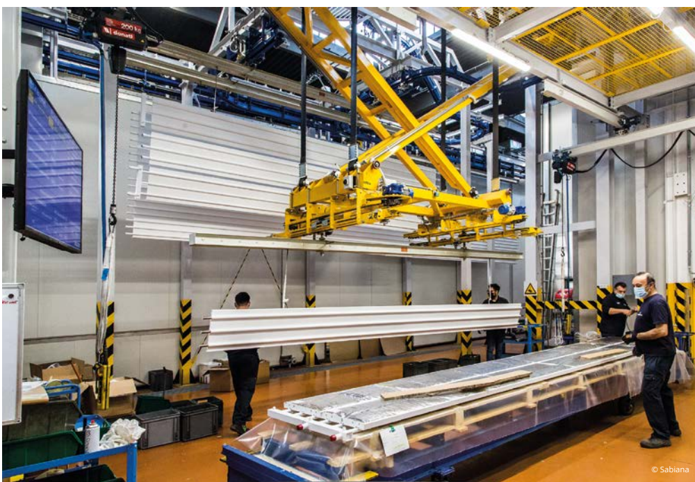
The unloading station with a lowerator.
