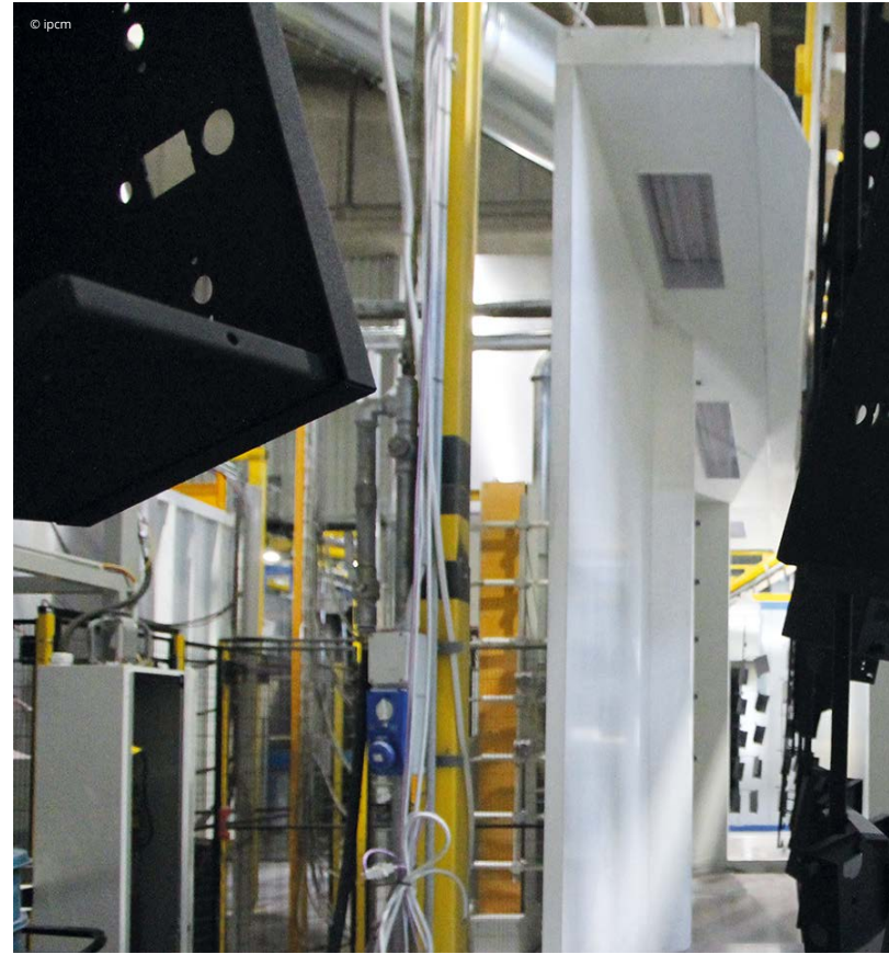
The second powder coating booth equipped with traditional Venturi technology and a second articulated robot for the pre-retouching operations.
