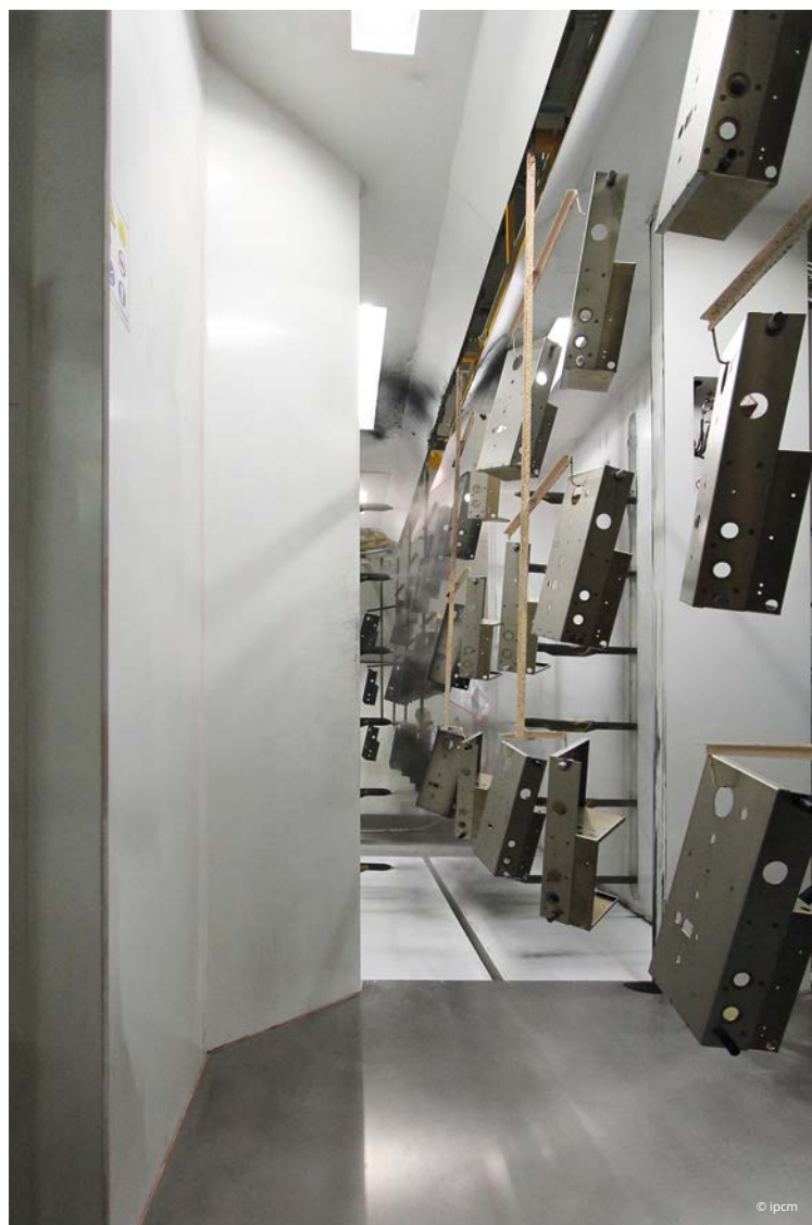
Application of the powder coating with dense phase technology.
