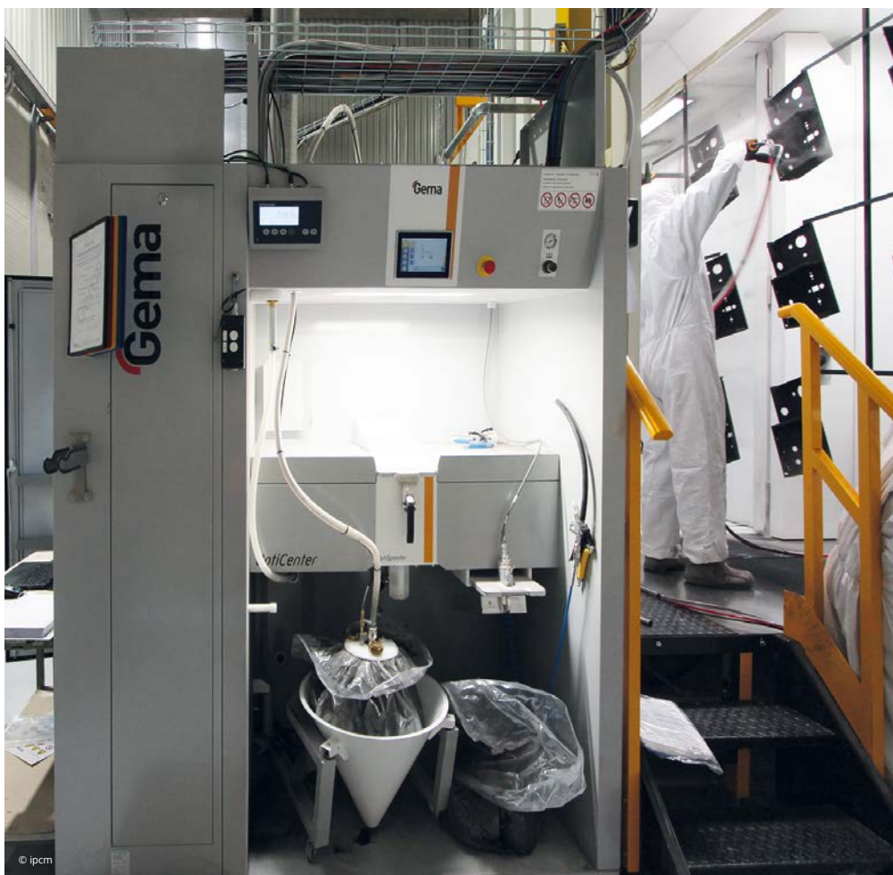
One of the two powder centres by GEMA and, on the right, the articulated robot by Lesta for the pre-retouching installed at the entrance of the dense phase coating booth.
