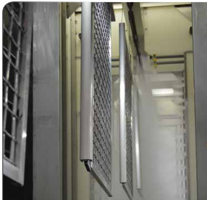
The automated washer process in Stage 1 has the Coral Clene 5011 acid cleaner and deoxidizer, reverse osmosis rinses in Stages 2 and 3, and Coral's Cor Bond Al non-chrome treatment in Stage 4.
