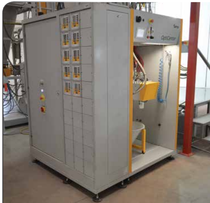
The Gema Magic System was installed to handle the coating side of the system, which includes the OptiCenter, ZA reciprocators, eight OptiGuns and CM touchscreen controls that are all designed to work together for quick and clean color change.
