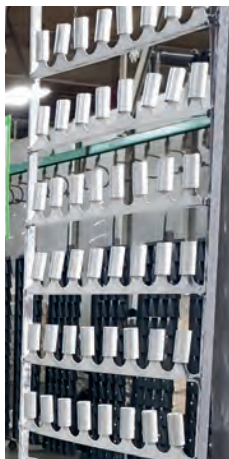
Maximizing rack density and ensuring your parts are presented properly to the powder guns is a critical first step in developing repeatable processes.
