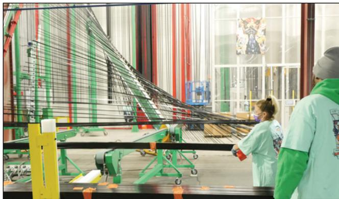
Figure 3. Personnel at the Garden City plant monitor the coated extrusions as they come off the new CUBE vertical powder coating line.
