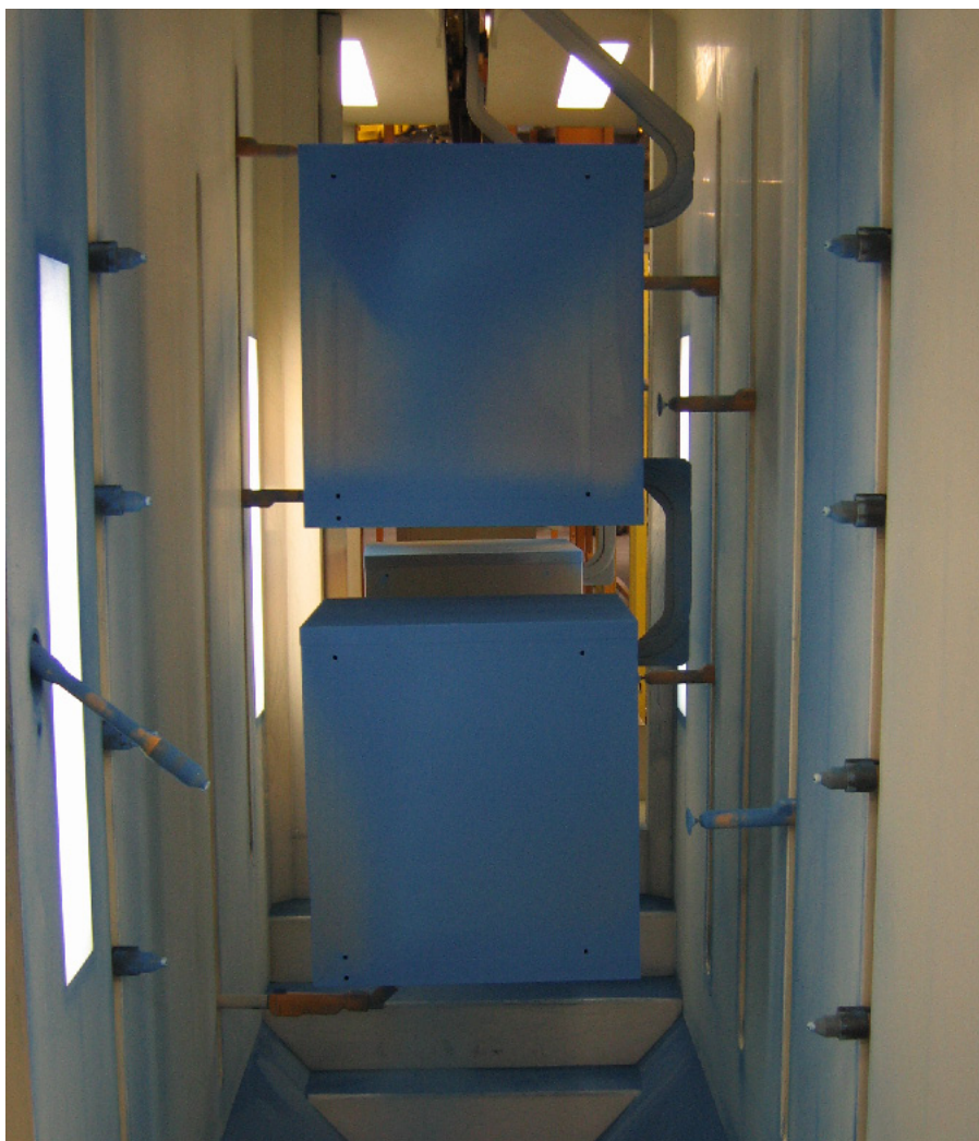
The gun configuration and the use of various kinds of independent axes allow simultaneous coating of the lower and upper parts of the cabinets hung on double hangers.
