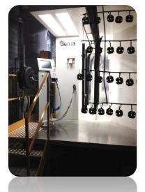
Previously equipped only with a manual installation, the company sprayed 55 to 60 tons of powder per year on its production of medical beds and hospital equipment. With 25% of wasted powder, the main aim was to develop a way to save powder, keep a constant quality and an efficient automation.
