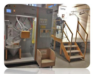
decided to change for a brand new Gema automatic booth system. The MagicCompact BA04 equipped with 6 GA03 automatic guns, 1 powder management OptiCenter OC02, coupled efficient with the powder recycling Gema system has been adjusted with two manual coating platforms, for pre and post touch-up. After reaching perfect settings,
